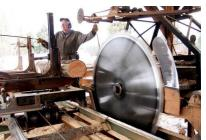
3. When at the sawmill, machines such as band saws and circular saws are used to create boards/planks.
