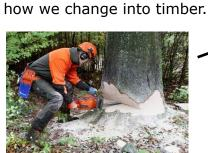
1. When trees are cut down, this is known as **felling.** This can be through machine or chain saws, just like the image.
